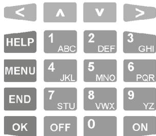
The DIGIT keys are used for entering your secret PIN code. You have 10 seconds to enter each digit, and must press the <OK> key when complete. This sequence is required before any panel operations can be performed. These keys can also be used to search for an item to be controlled by selecting the first letter of it's name.
